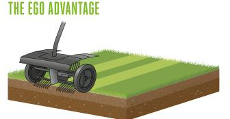
**Competitor Dethatchers** Separated cylinders cause missing area in the middle
